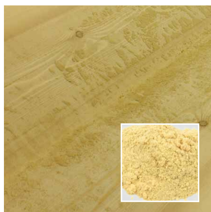
Saw dust accumulation with standard saw blade
