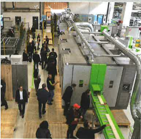
Fully automated softwood production line for multi-layer boards draws the crowds.
