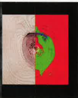
The result of hyperspectral imaging is shown on the right; in this case, a growth defect (knot)
