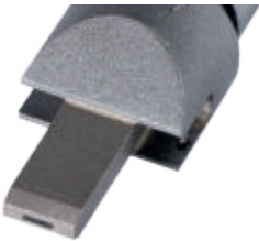
Diamond dresser Square 1 x 0,4 x 2,0 mm, Total bearing surface 0,80 mm 2 , r = 0,21 mm
