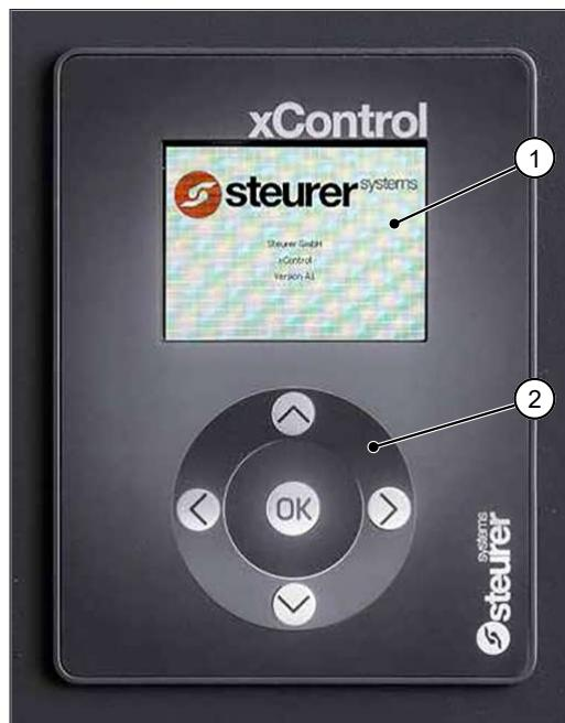
The following start-up screen appears once the device has been switched on.
