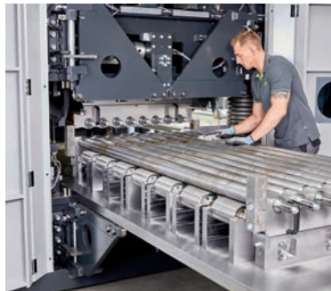
Advanced cleaning system for leveling rollers
