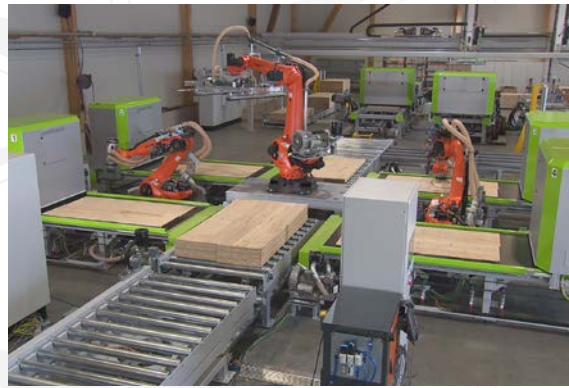
Fully automatic cleaning and repair of panels
