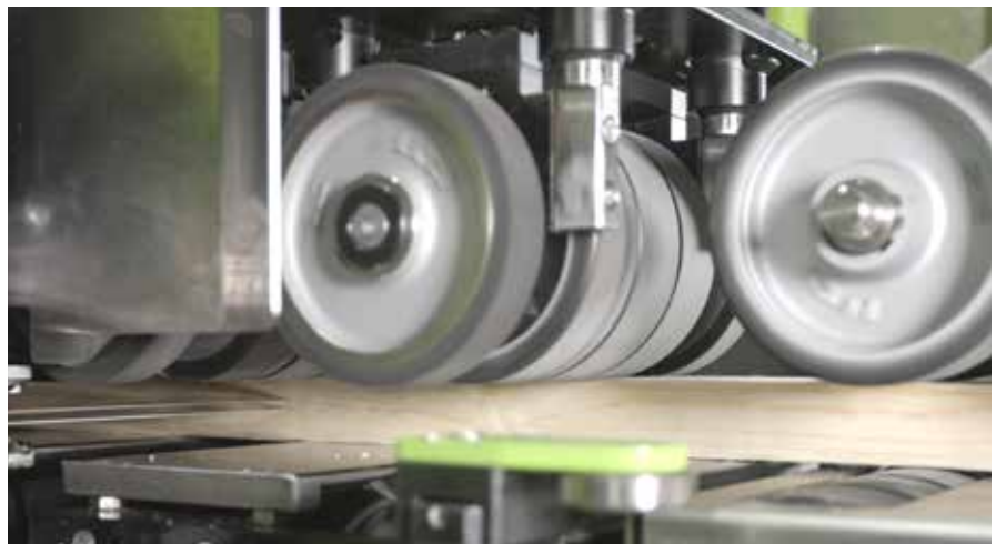
Driven feed rollers top and bottom
