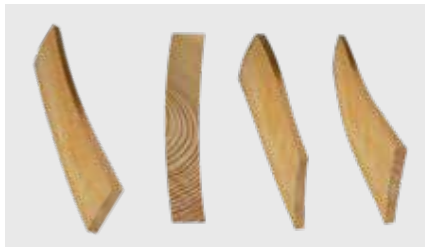
Blocks with longitudinal/latitudinal deformation, cupped or warped
