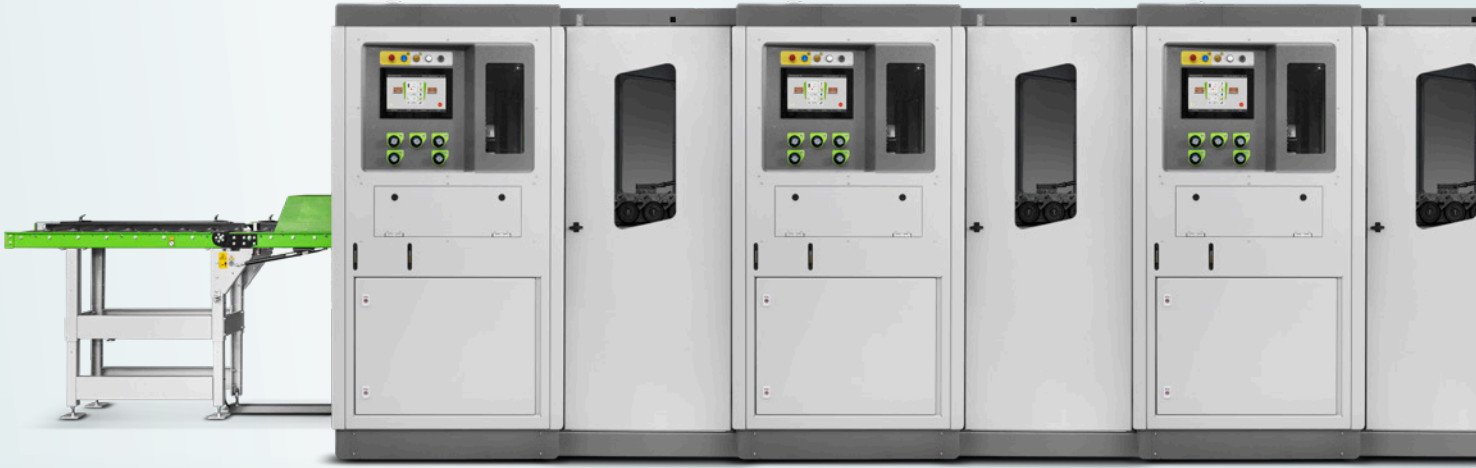
6 DSB Singlehead Pro XM connected in series with a total of 6 saw modules
