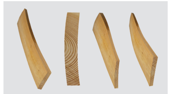
Blocks with longitudinal/latitudinal deformation, cupped or warped
