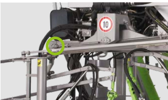
Screws on the rear axle for adjusting track width
