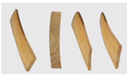
Blocks with longitudinal/latitudinal deformation, cupped or warped
