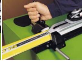
**Clamping.** The new **speedtronic's** clamping system with laser positioning drastically reduces the handling effort: positioning and clamping are carried out in no time! Whether alpine or carving skis - the **speedtronic** enables all ski widths and surfaces to be clamped and offers easy access to adjust the bindings.
