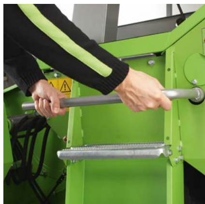
Threshing drum reversing mechanism
