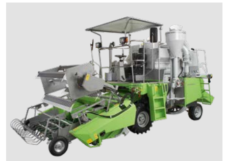
Delta with tine cloth pick-up device
