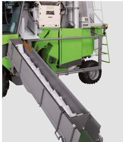
Adjustable height for emptying the sample conveyor belt
