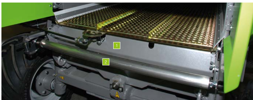
1 Electrical adjustable sieve setting 2 Grain loss sensor
