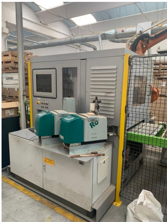
TRC 1000 - fully automatic wood surface repair plant
