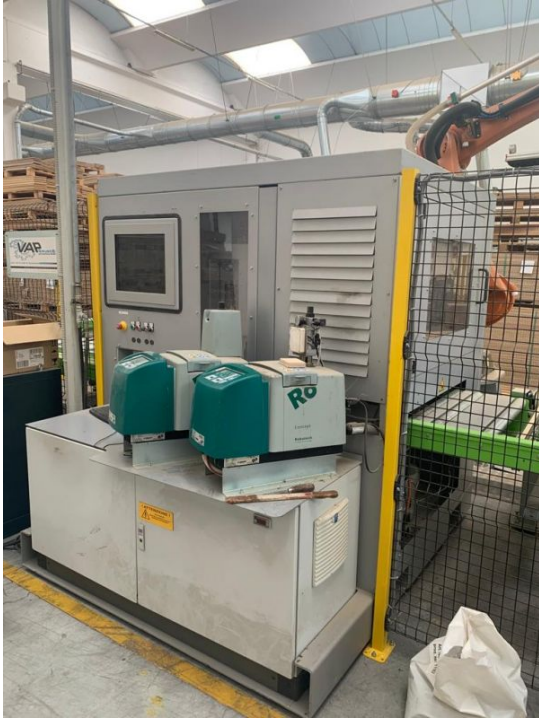
TRC 1000 - fully automatic wood surface repair plant
